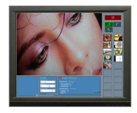
For particular points of interest on the web Fusion-DX offer its users the ability to easily store the position and zoom setting of those points along with a **Thumbnail** image. Up to 18 Thumbnails can be stored per Job, and the camera position for any Thumbnail can be quickly recalled by simply touching the appropriate Thumbnail on screen.
